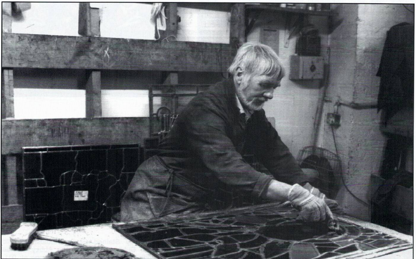
Cement putty is forced into the lead.
